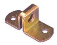
Made from heavy-gauge steel and pre-drilled for assembly with two 1/4" bolts. Smaller version of the 1/2" Shackle Plate<sup>TM</sup> that will mount easily and more discreetly into the bottom-rail of any wood or metal fl at, and can also be used as a fl oor or ceiling plate.
